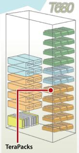
Spectra's TeraPack® tape containers streamline loading and unloading, handling 9 TS\* or 10 LTO tapes at once.
