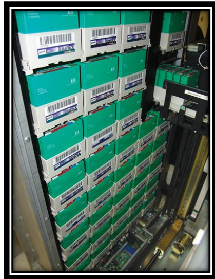
Figure 10: Spectra Enterprise Library Terapack Architecture
