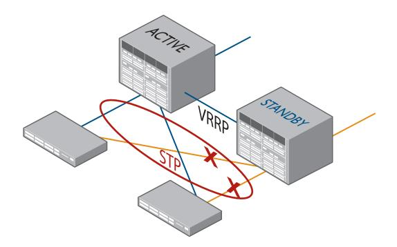
The above diagram shows how STP blocks links to prevent loops, but causes reduced bandwidth.
