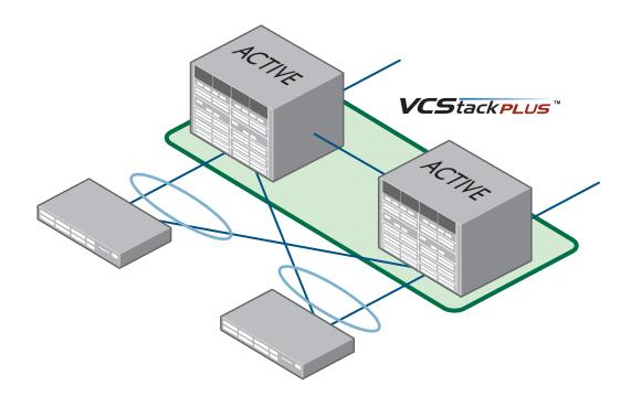
This diagram shows how a stacked system allows all links to remain active. LAGs can be configured across both chassis because they belong to the stack and are treated as a single virtual device. Bandwidth is maximized and recovery from link failures is almost instantaneous. For time-critical applications, using LAGs helps to reduce latency – traffic can always follow the most direct path because no links are blocked.
